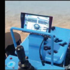
Video telecamera posteriore Rear view video camera to view sieve
